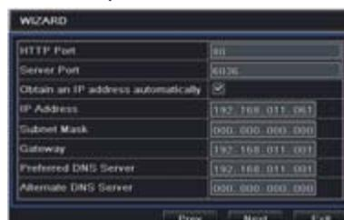
The default HTTP port is 80. The default server port is 6036. You can check 'Obtain an IP address automatically' to acquire network information or input IP address, subnet mask, gateway, preferred/alternate DNS server manually. This function is used to monitor DVR through internet (See Section 10 for details).
