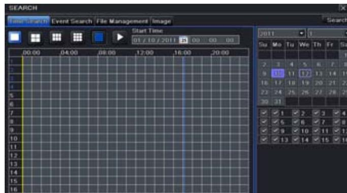
Step 2: Select date and channels on the right hand side and press "Search" button. A date with highlighted borderline indicates presence of data.
