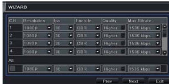
Select resolution, fps, encode, quality and bitrate. The higher the value is, the clearer the recorded picture is. Of course, more space of HDD will be taken up.
