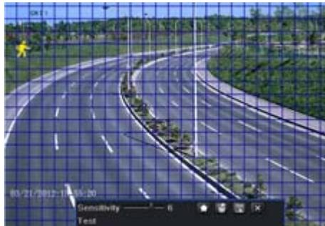
Step 5: Enter into Menu→Setup→Alarm→Motion→Schedule tab to bring up schedule settings for motion alarm. The setup steps are similar to normal schedule setup. You can refer to 7.2 Schedule Recording for details.
