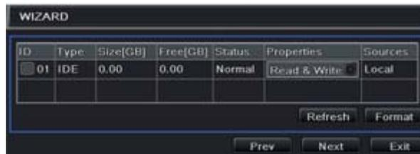
You can check your HDD information through this tab. If your HDD was recently installed, select the HDD from the list to format it.
