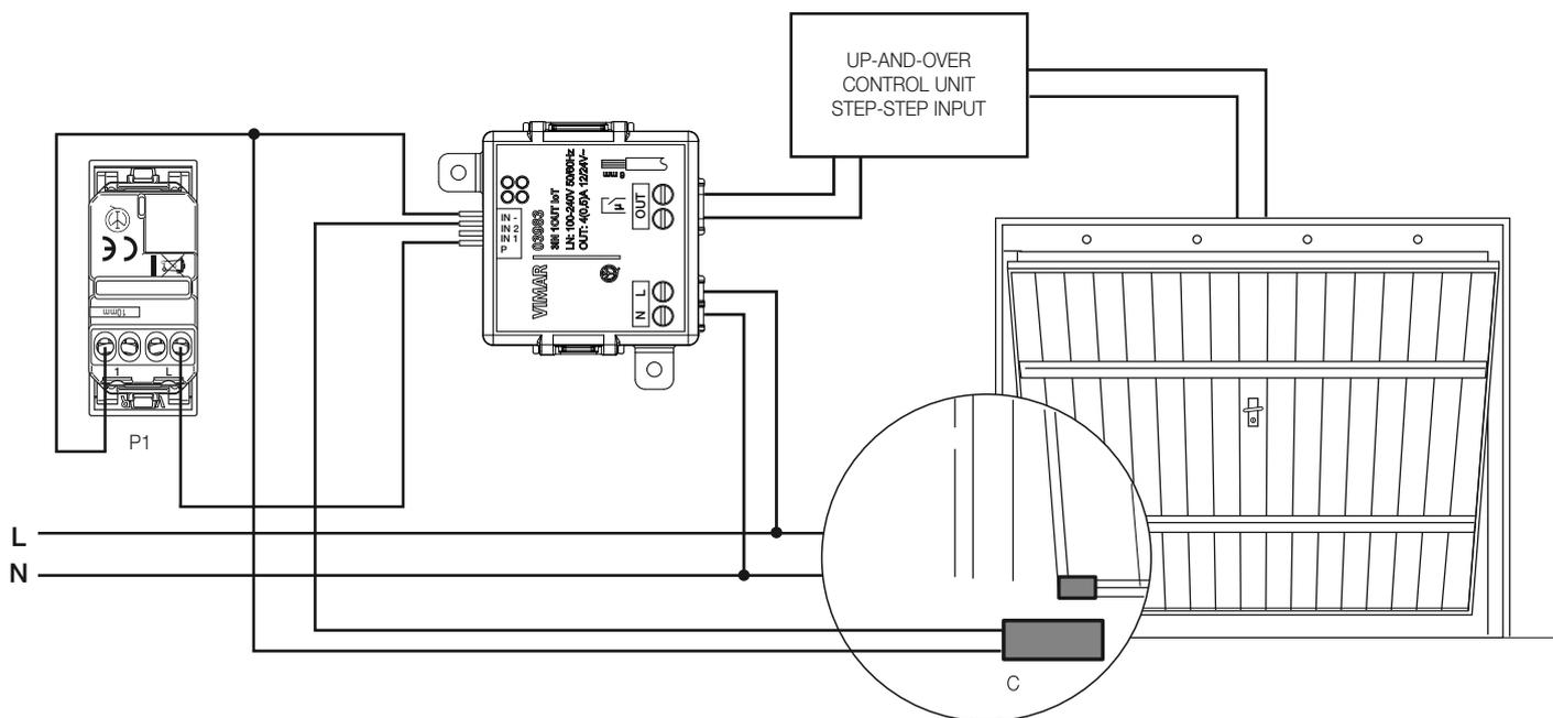
C: Magnetic contact for protecting up-and-over doors, sectional doors, roller shutters (art. 01824).
