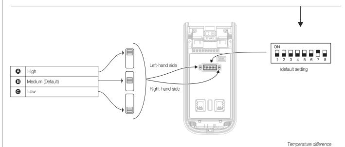
\* Alarm outputs; ON/OFF of individual outputs via DIP switch No.3
