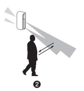
Check whether the LED flashes for 2 seconds when the desired object is detected
