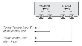
(\*) Generally speaking the roller shutter/inertia detectors do not have a terminal dedicated to sabotage/tampering.
