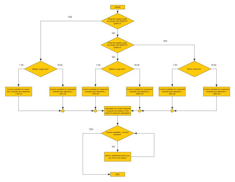
CAUTION: For the correct sizing of the system, always consider the maximum consumption condition; this condition varies according to the number of devices present in the system and to the configuration created.
