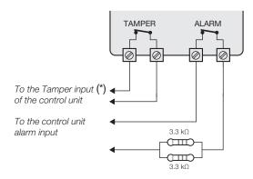
(\*) Generally speaking the roller shutter/inertia detectors do not have a terminal dedicated to sabotage/tampering.
