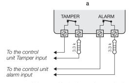
To the control unit alarm input
