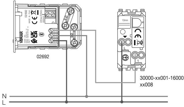
2. Collegamento a lampada spia • Connection to the pilot lamp
