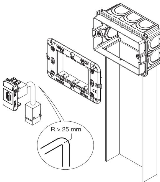
**INSTALLAZIONE DA INCASSO • INSTALLATION FLUSH-MOUNTING • INSTALLATION D'ENCASTREMENT
