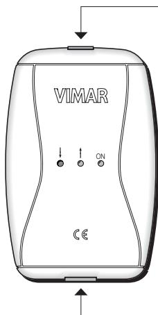
Connettore USB (PC EasyTool Professional o Configuratore touch screen Well-contact Plus)
