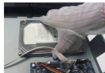
3- Place the HDDs onto the bottom of the machine.
