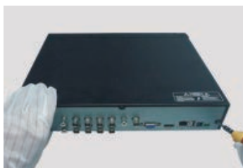
1- Loosen the screws to open the cover.
