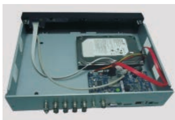
4- Connect the power and data cables.
