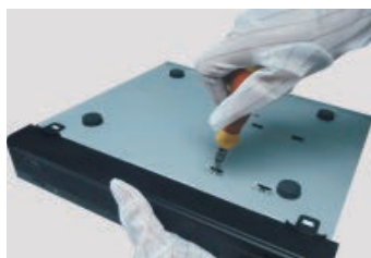
5- Turn over the machine and secure the HDDs.
