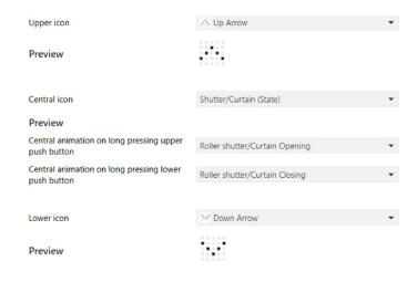
"Definition of the LED matrices for the switching module" parameters
