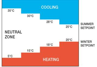
CAUTION: When the thermostat is in Neutral Zone mode, the breadth of this must be progressively increasing for the different operating modes of Comfort (minimum neutral zone breadth), Standby, Energy Saving and Protected. This setting made with ETS ensures that, when the thermostat changes operating mode, the active setpoint is always at a suitable value and the thermostat does not start cooling if it was heating before or vice versa, causing considerable energy consumption. Continued
