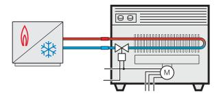
Installation of 4-pipe fan coil solenoid valve
