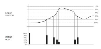
The parameters of the proportional and integral coefficients Kp and Ki are set using the ETS software: the proportional coefficient Kp for heating corresponds to the "Heating Proportional Value" parameter while the coefficient for cooling is set using the "Cooling Proportional Value" parameter. The integral time Ti is set with the "Heating Integral Value" and "Cooling Integral Value" parameters for heating and cooling, respectively.
