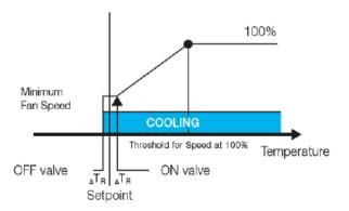
N.B.: Fore reasons tied to the safety of systems, if the valve is active the user will be unable to set "OFF" from the thermostat. It will therefore be necessary to turn off the valve by setting the thermostat to another mode or by modifying its setpoint.
