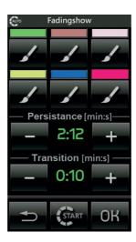
The function of Fading-Show allows to set a cyclical sequence of colors (up to a maximum of 6) for color changes and the play of light in the environments where the lamps are installed RGB.
