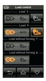
Tapping the icon corresponding to the desired load, forces that load.
