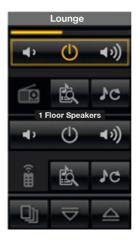
This screen is used to control switching the audio zone on/off and adjusting the volume.
