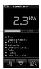
• Tapping displays the screen with which you can force the loads.
