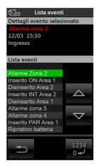
The screen for the event list allows <u>displaying the last 32 events saved</u> by the video touchscreen (use the and icons to scroll through the list and the icon to clear the list) consulting the characteristics of each event (type, date and time, zone/area details) in the **Dettagli evento** column.
