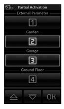
To include an area in partialization, it is sufficient to touch the corresponding icon and the edge of the latter will become yellow in colour.
