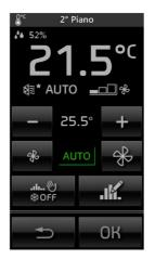
• Via soft you can view the screen for setting AUTO, MANUAL, REDUCTION, AWAY and PROTECTION operation (Antifreeze or TooHot depending on the seasonal mode) of the heating/air conditioning system.
