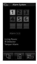
The touch screen allows the burglar alarm system to be switched on/off with modes similar to those of the digital keypad and therefore by typing in PIN codes; the screen is as follows:
