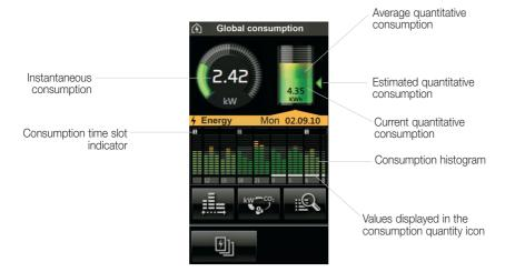
**Dynamic Mode:** Pressing the area that displays the instantaneous power for 2 min after the reading of the will value every 2 s thus increasing the frequency of update of the data represented. At the end of 2 min, the reading will repeat every 30 seconds until an eventual new pressure.
