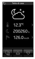
The arrows next to the temperature and wind speed take you to a page showing the extreme values recorded. Resetting these values can be done manually (with the specific button) or automatically at midnight every day. The choice between the two reset modes is made during installation.
