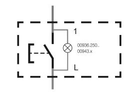
When pressing the control push button, the visible in darkness pilot light switches off.
