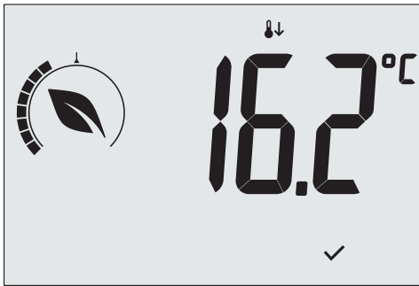
Fig. 9: Input in Nighttime Reduction mode showing the reduction set point
