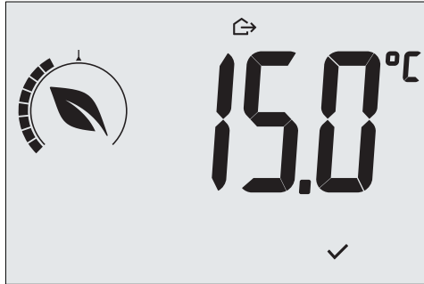
Fig. 7: Input in away mode showing the away temperature
