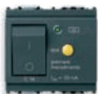
16511.16 C 16, I_{\Delta n} 10 mA, prekidna moć 3000 A - 2 modula. Dubina: 38 mm
