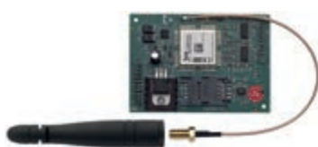
01706 Modul predajnika/prijamnika GSM Dual Band GSM/GPRS 900/1800 MHz
