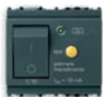
16511.10 C 10, I_{\Delta n} 10 mA, prekidna moć 3000 A - 2 modula. Dubina: 38 mm
