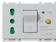
14283.SL Bpresa 16 A P17/11 250 V~, 1P+N C 16 - 3 modula
