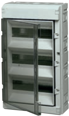
V51136 36 modules, with adjustable DIN rail (60715 TH35) to accommodate non-standard products, RAL 7035 grey, with transparent door and screwcaps for double insulation. Dissipated power: 32 W
