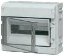
V51112 12 modules, with adjustable DIN rail (60715 TH35) to accommodate non-standard products, RAL 7035 grey, with transparent door and screwcaps for double insulation. Dissipated power: 21 W
