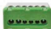
V53552.V Screw terminal block with 6 holes for consumer unit, to insert cable conduits from 1,5 mm 2 to 16 mm 2 diameter, snap fixing to the terminal block support, green
