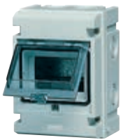
V51005 5 (4+1) modules, with screwcaps for double insulation, with DIN rail (60715 TH35), RAL 7035 grey, with transparent door, fumé. Pre-set for 2 supports for earth terminal blocks V51853. Dissipated power: 12 W
