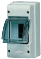
V51003 3 (1+2) modules, with screwcaps for double insulation, with DIN rail (60715 TH35), RAL 7035 grey, with transparent door, fumé. Dissipated power: 9 W
