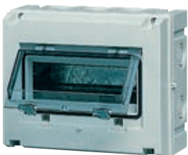
V51008 8 modules, with screwcaps for double insulation, with DIN rail (60715 TH35), RAL 7035 grey, with transparent door, fumé. Dissipated power: 21 W
