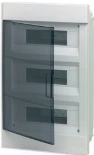
Δ V52436 36 modules, delivered with DIN rail (60715 TH35), RAL 9003 white, with transparent door, fumé. Dissipated power: 68 W
