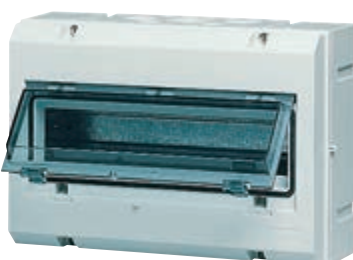
V51012 12+1 modules, with screwcaps for double insulation, with DIN rail (60715 TH35), RAL 7035 grey, with transparent door, fumé. Dissipated power: 26 W
