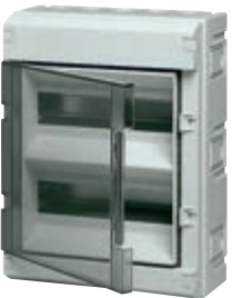
V51124 24 modules, with adjustable DIN rail (60715 TH35) to accommodate non-standard products, RAL 7035 grey, with transparent door and screwcaps for double insulation. Dissipated power: 27 W
