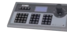
Δ 46916.001 RS485 keypad for PTZ control and DVR management, multi-protocol, 8 devices in cascade (in-out) 4-line display, 3-axis control, 12V power supply unit.
