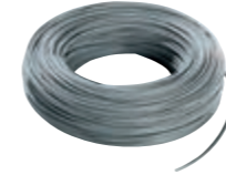
0002.060.E 75 ohm coaxial cable, cable ø 3 mm, with PVC sheath, CPR Eca class, suitable for installation with Category I power cables (U0 = 400 V), grey - 200 m spool
