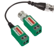
46862.B02 Pair of passive video transducers for video transmission over twisted pair, BNC connector for connection to the camera or DVR, one transducer with 14 cm of cable, screw connection for the cable
