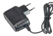
46902.010 Switching-mode power supply unit, 100 – 240 Vac 50/60 Hz, integrated Europlug 2P plug, output with standard jack connector 12 Vdc 1 A, maximum power 12 W
