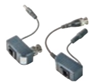
46862.B01 Pair of Balun passive video transducers (transmitter/receiver) for video transmission over twisted pair, BNC connector for the video, jack for the power supply, cable connection with RJ45 connector, maximum distance attainable with Cat. 5 cable 50 m, compatible with PAL/NSC/SECAM, built-in electrostatic discharge protection
