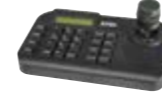
46916.005 Control keypad for Speed Dome cameras, with 3-axis Pelco D, Pelco P Protocol, standard 12 Vdc 2 A power supply unit. Dimensions: 220x130x90 mm
