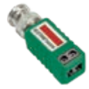
46862.001.01 Balun video passive transducer for video transmission over twisted pair, BNC connector for connection to the camera or DVR, screw connection for the cable
