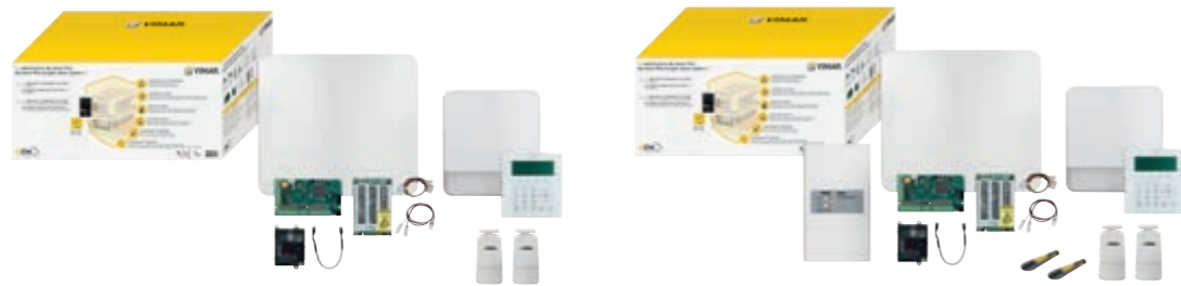
▲ 0K03800.02 By-alarm Plus control unit kit, 25 zones , surface mounting, containing: • 1 25-zone control unit board (03800) • 1 keypad with display (03817) • 1 outdoor siren (03827) • 2 dual technology surface mounting detectors (01721) • 1 burglar alarm system gateway (03812) • 1 230 V – 13 Vdc 3.2 A power supply unit (03805) • 1 plastic box (03814)
