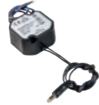
46901.015 Flush mounting switching mode power supply unit, 100 – 240 Vac 50/60 Hz power supply, 12 Vdc 1.5 A output with standard jack connector, maximum power 18 W, installation in switchboards, junction boxes or watertight enclosures
