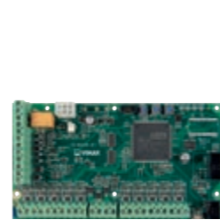
▲ 03801 By-alarm Plus control unit expandable to 65 zones
