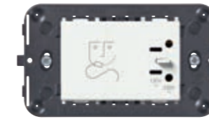
09290 Shaver supply unit with 20 VA isolating transformer, 230 V~ 50/60 Hz, 230 V~ and 120 V~ outputs - 3 modules. Depth: 42 mm
