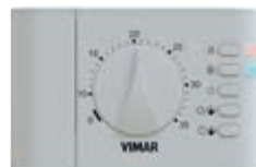
02900.1 Electronic thermostat for ON/OFF ambient temper- ature control (heating and air-conditioning), class I temperature control device (contribution 1%), change-over relay output 5(2) A 240 V~, AA LR6 1,5 V battery-powered (not supplied), surface mounting, white
