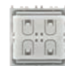
03925 Flat control with four push buttons with 2.4 GHz radio frequency transmitter, Bluetooth Low Energy standard, energy harvesting power supply provided by the built-in electro-dynamic generator, 2 modules.
