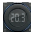
09470.CM Rotary dial thermostat for ambient temperature control, 5(2) A 240 V~ relay output, heating and air-conditioning ON/OFF, class I temperature control device (contribution 1%) in ON/OFF mode, white LED backlighting and brightness regulation, 100-240 V 50/60 Hz - 2 modules. Depth: 28,5 mm
