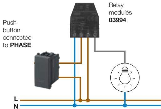
Connection of ON/OFF push button with **NEUTRAL**
